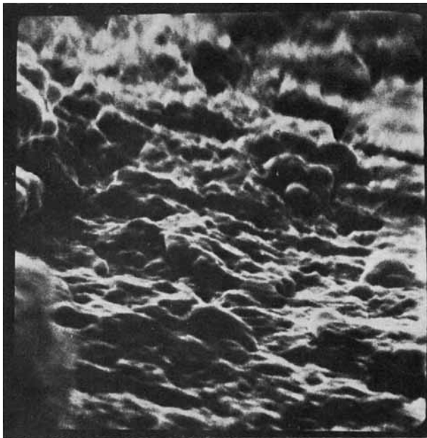
Fig. 11. Fracture surface stereoscanning electron micrograph ( \times 9,300 ) of SPVC sample milled at 220^{\circ}\text{C} .
