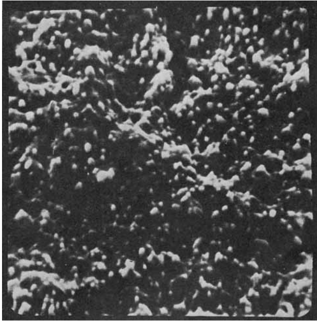
Fig. 6. Fracture surface stereoscanning electron photomicrograph ( \times 8,300 ) of commercial PVC sample milled at 140^{\circ}\text{C} .
